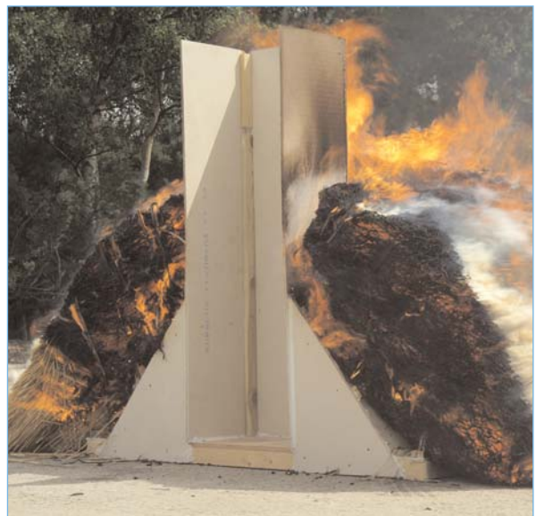
SUPALUX® – thatch fire test
